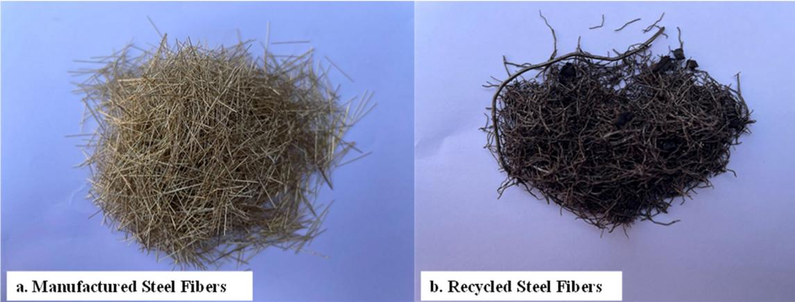
**Figure 2.4** Visual comparison of samples from manufactured steel fibers and recycled tire fibers
