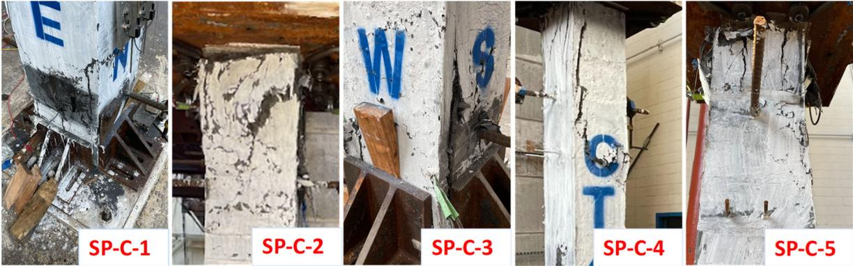
Figure 4.14 Mode of failure and damage pictures of the five tested Type C columns
