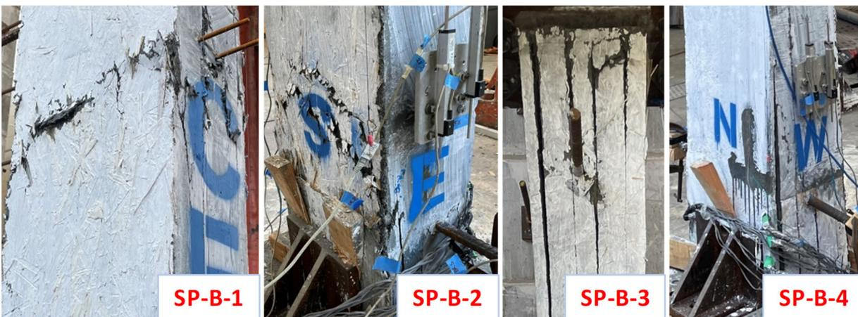
**Figure 4.7** Photographs of the Type B UHPC columns failure after axial testing
