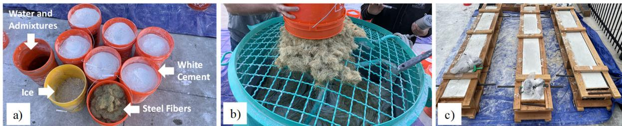
**Figure 2.1** (a) UHPC Type A ingredients; (b) illustration of adding the steel fibers into the mixture; and (c) photograph of sample cast UHPC Type A columns (horizontally positioned)
