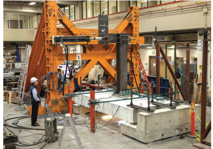
Moment transfer test specimen design and experimental setup
