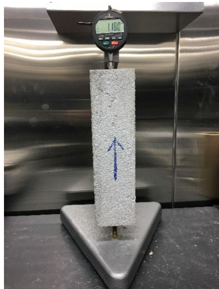
Figure 35 Length comparator used for shrinkage measurement
