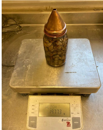
Figure 6 Aggregate absorption rate test setup
