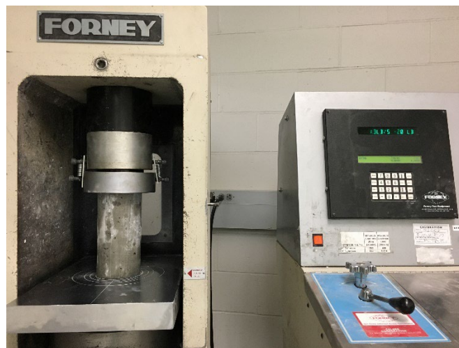
Figure 32 Compressive strength test setup
