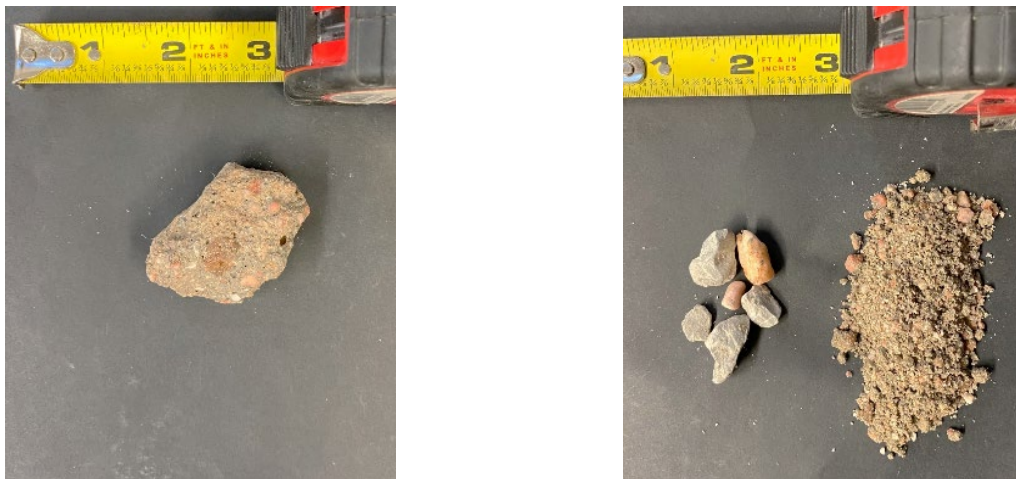
Figure 13 Example of RCA mortar disintegration after temperature shock
