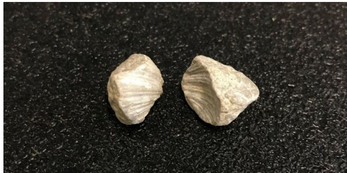
Figure 20 Example of natural aggregate becoming too brittle
