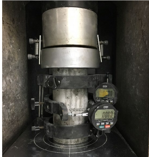
Figure 33 Static modulus of elasticity test setup
