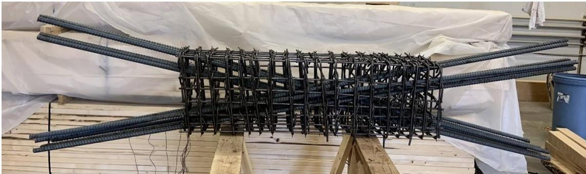
Figure 4.9. Reinforcement Cage for D(#6)-3.0-0.69 or D(#6)-3.0-1.38
