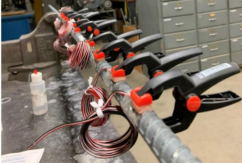
Figure 4.5. Strain Gauge Installation
