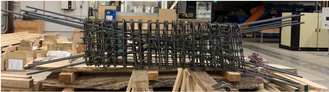
Figure 4.8. Reinforcement Cage for D(#4)-3.0-0.69 or D(#4)-3.0-1.38
