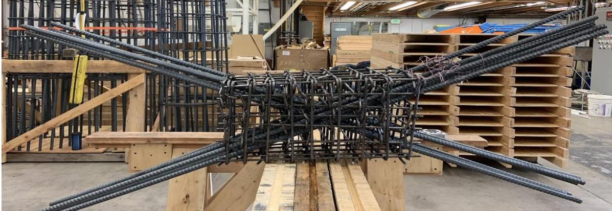
Figure 4.10. Reinforcement Cage for D(#6)-1.5-0.69
