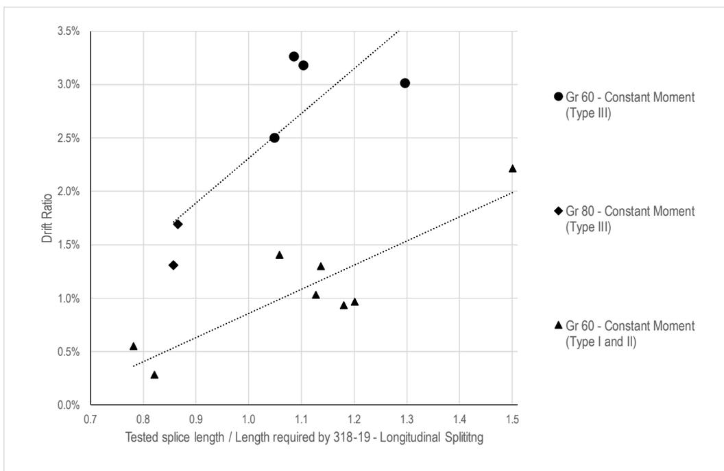
Figure 64 – Variation in Drift Ratio at Failure with Increases in Ratio of Length of Lap Splice to Length Required by ACI318-19 Formulation Used Assuming Longitudinal Splitting Controlled.
