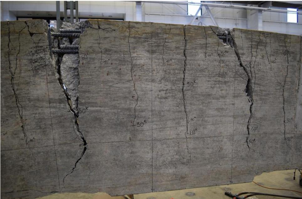
A photograph showing the failure of test beam WB60U1. The beam is a concrete slab with several horizontal reinforcement bars. The failure is characterized by a large, jagged fracture along the lap splice, with significant concrete spalling and exposed steel bars. The beam surface is marked with handwritten annotations, including "30k", "40k", "50k", and "60k", indicating load levels. The background shows a large industrial or laboratory setting with high ceilings and structural columns. |
