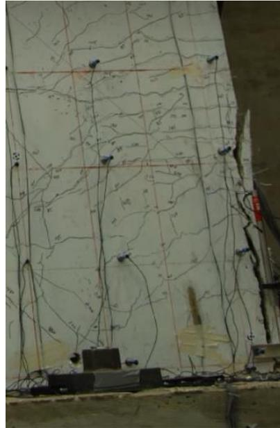
Figure 10 –Splitting cracks in lap splice in Specimen PW1 by Birely (2012).
