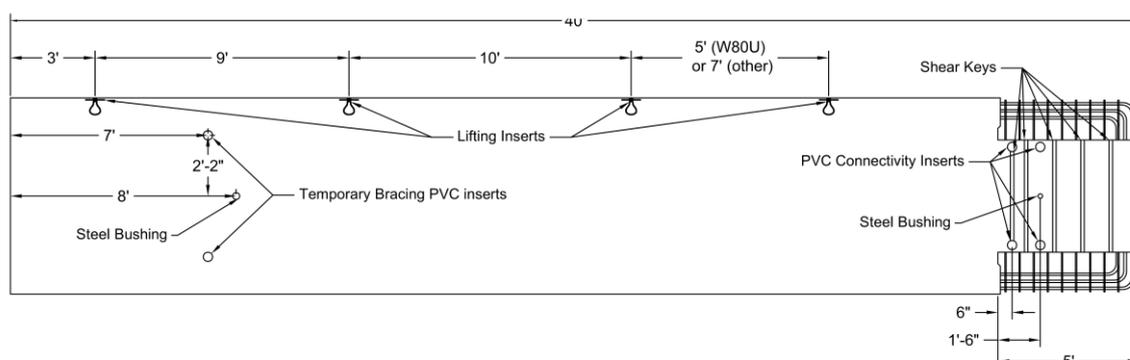
Figure 46 – Lifting Inserts and Openings in Test Walls.
