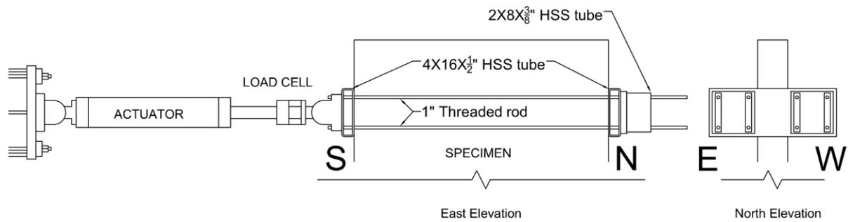
Figure 29 – Lateral Loading Rig
