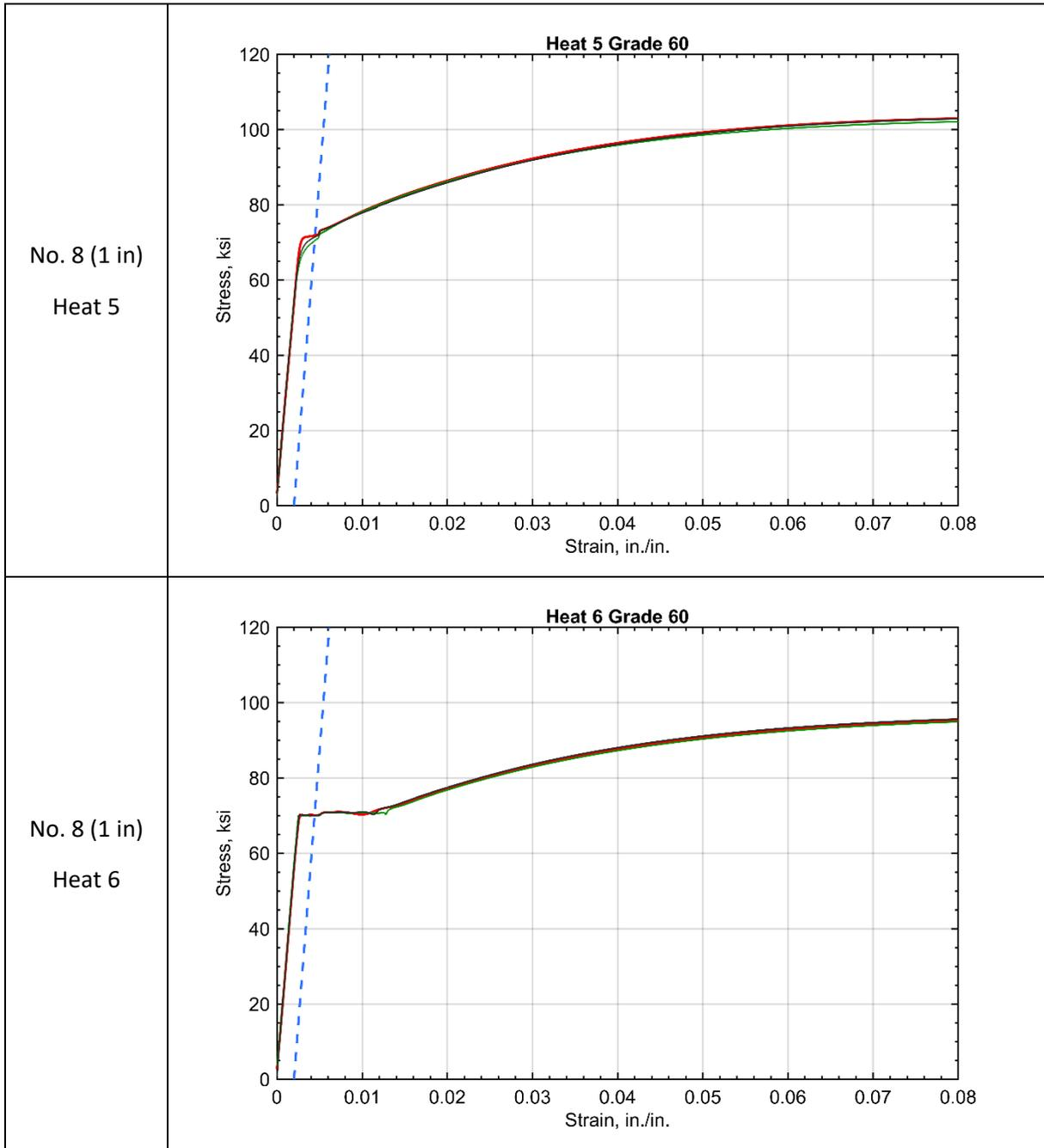
Figure 34 – Stress-Strain Curves Measured in Grade-60 Bars.
