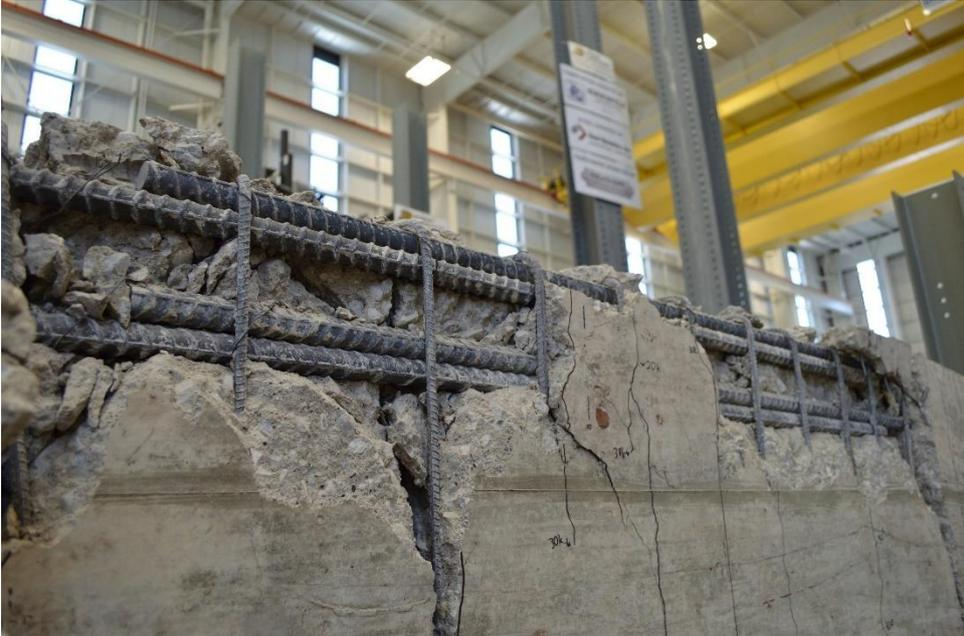
A photograph showing the failure of test beam WB60U0. The beam is a concrete slab with several horizontal reinforcement bars. The failure is characterized by a large, jagged fracture along the lap splice, with significant concrete spalling and exposed steel bars. The background shows a large industrial or laboratory setting with high ceilings and structural columns.                                                                                                                             |
