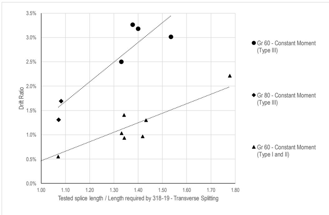
Figure 63 – Variation in Drift Ratio at Failure with Increases in Ratio of Length of Lap Splice to Length Required by ACI318-19 Formulation Used Assuming Transverse Splitting Controlled.
