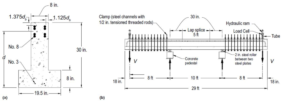
Figure 14 – Cross section and elevation, specimens by Richter and Hardisty (2012, 2015).
