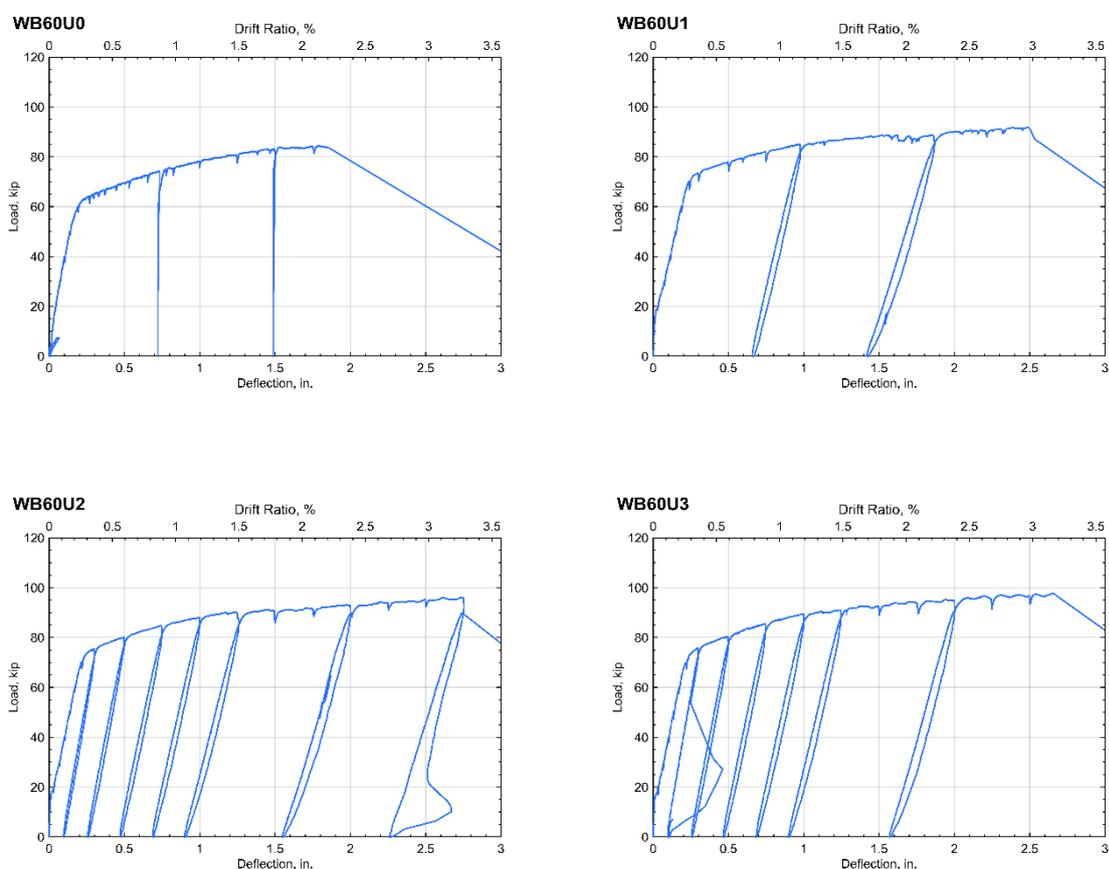
Figure 55 – Load-Deflection Relationships Measured in Test Beams.
