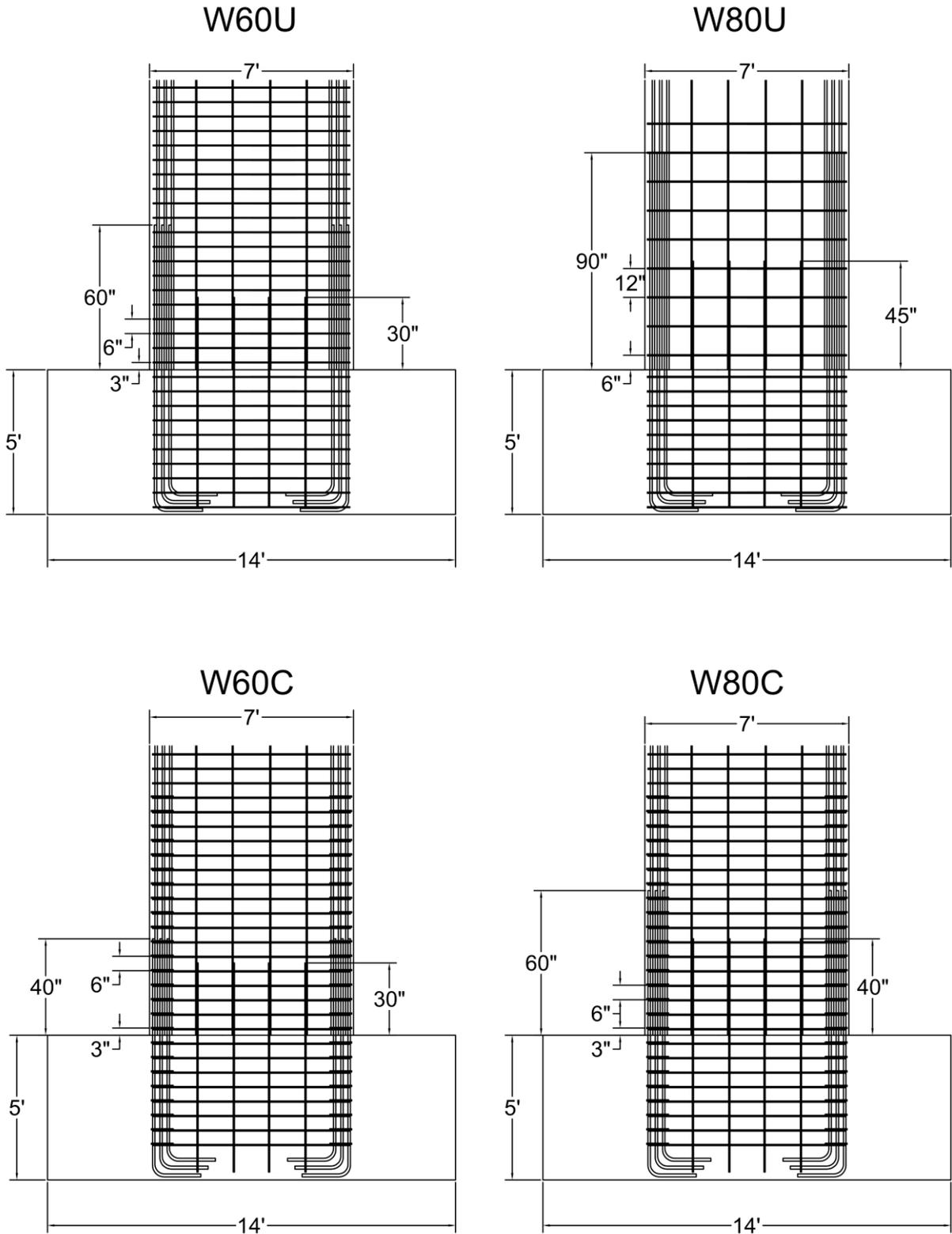
Figure 25 – Test Wall Partial Elevations
