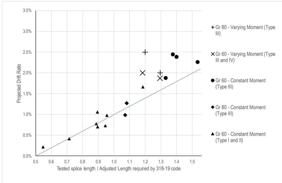
b) drift ratios measured in test beams at failure multiplied by 3/4
