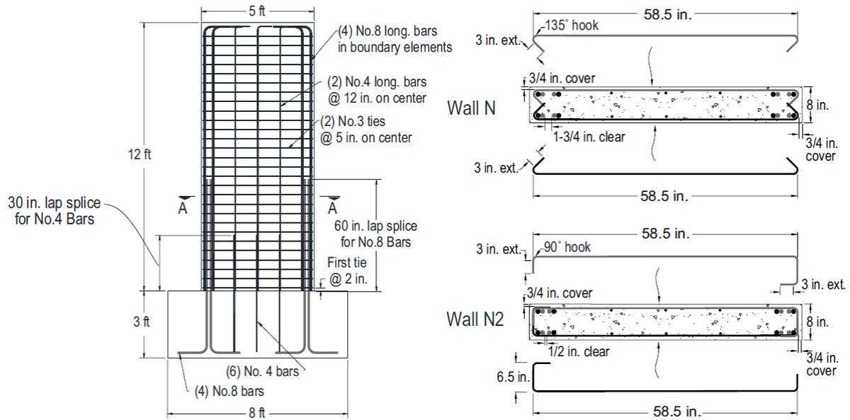
Figure 12 – Details of specimens tested by Villalobos (2014, 2017).
