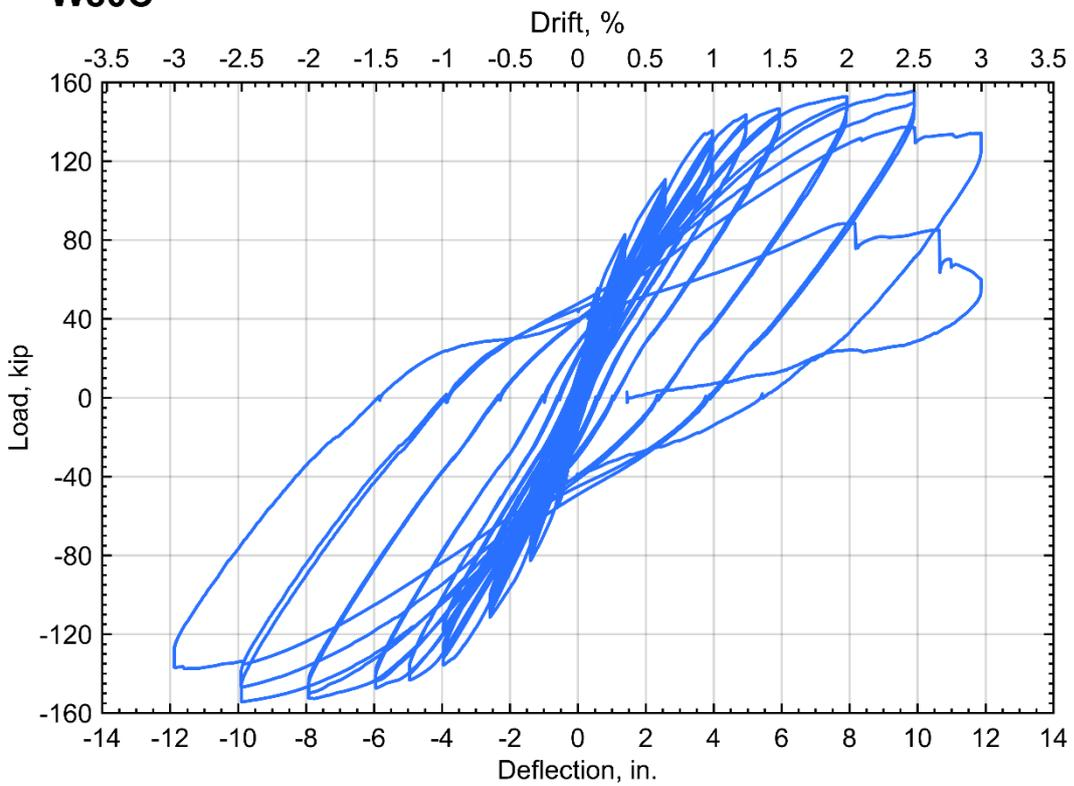
Figure 70 – Specimen W80C, Measured Load-Deflection Curve.
