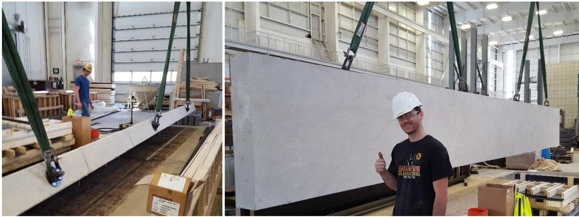
*Figure 40 – Tilt-up and transportation of test beam.*
