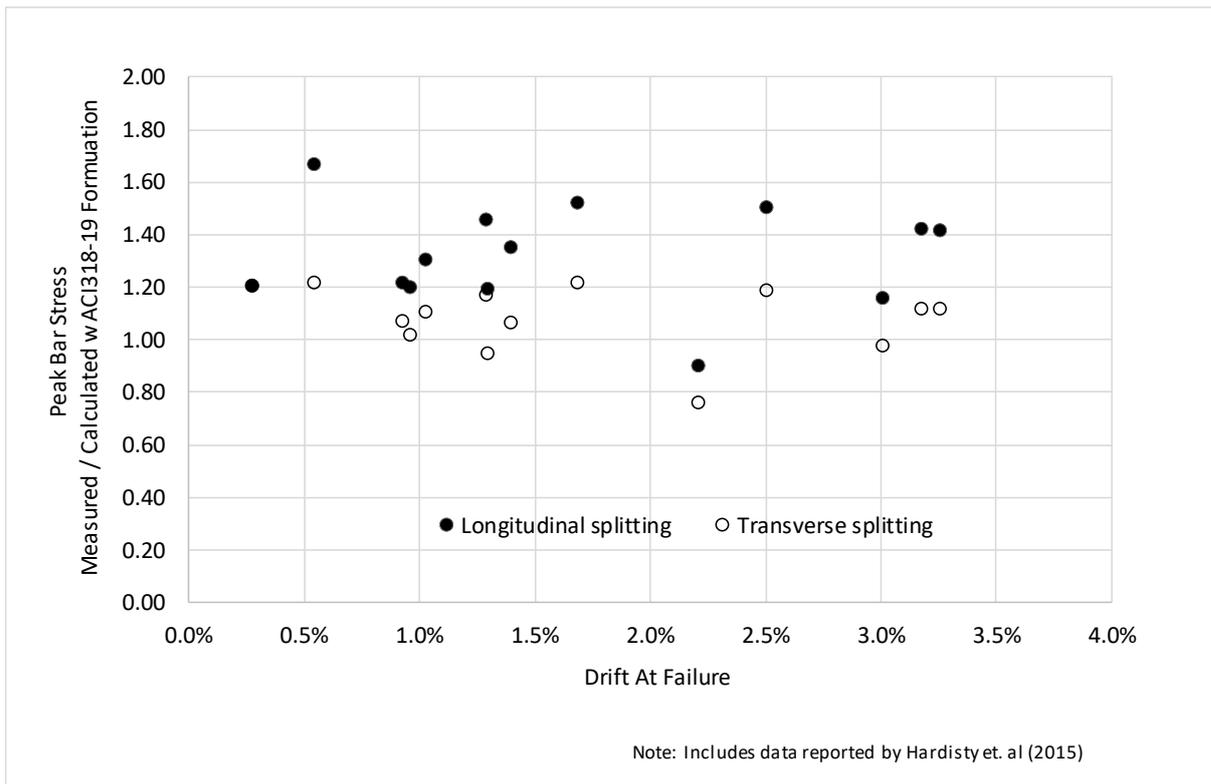
Figure 62<sup>8</sup> – Ratio of Measured to Calculated Peak Bar Stress - Formulation by ACI 318-19 (ACI, 2019).
