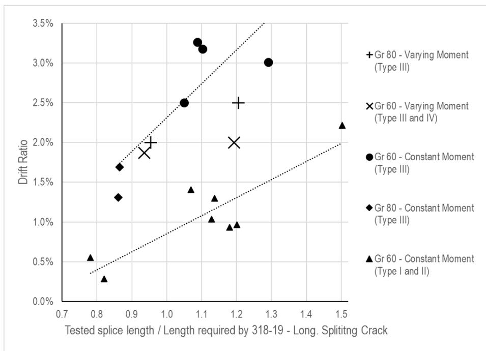
Figure 80 – Variations in Limiting Drift Ratio with Increases in Ratio of Length of Lap Splice to Length Required by ACI318-19.- Formulation Used Assuming Longitudinal Splitting Controlled
