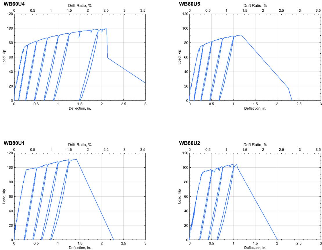
Figure 55 (Continued) – Load-Deflection Relationships Measured in Test Beams.
