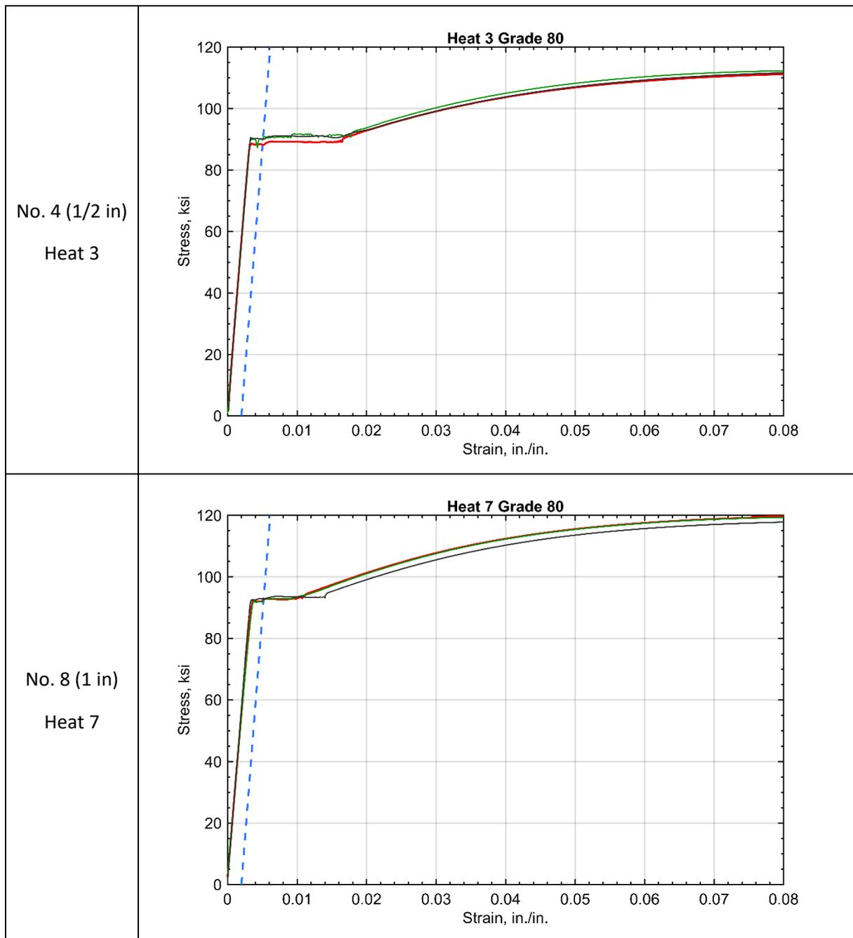
Figure 35 – Stress-Strain Curves Measured in Grade-80 Bars.
