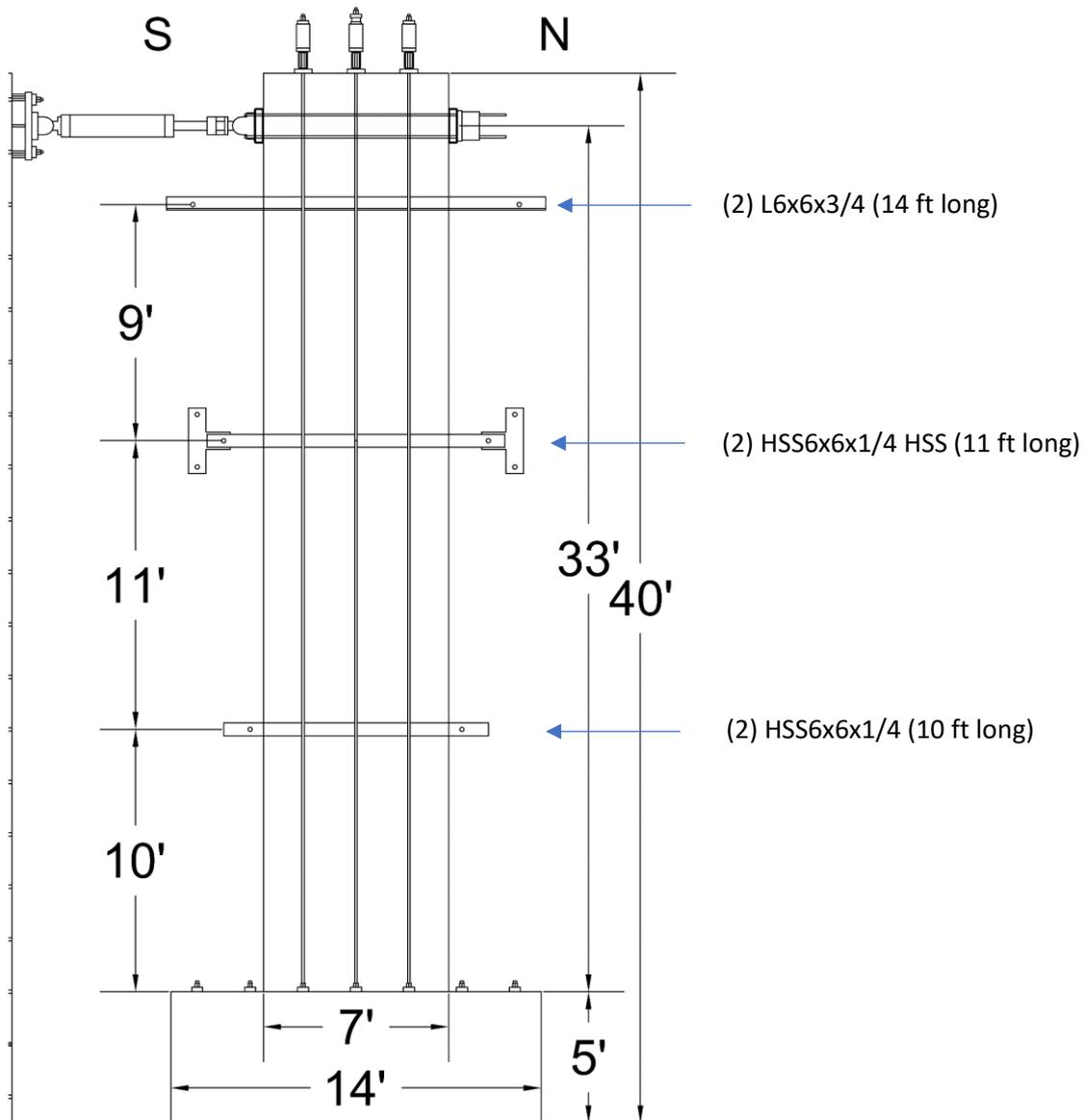
Figure 48 – Details of Bracing used for Test Walls.
