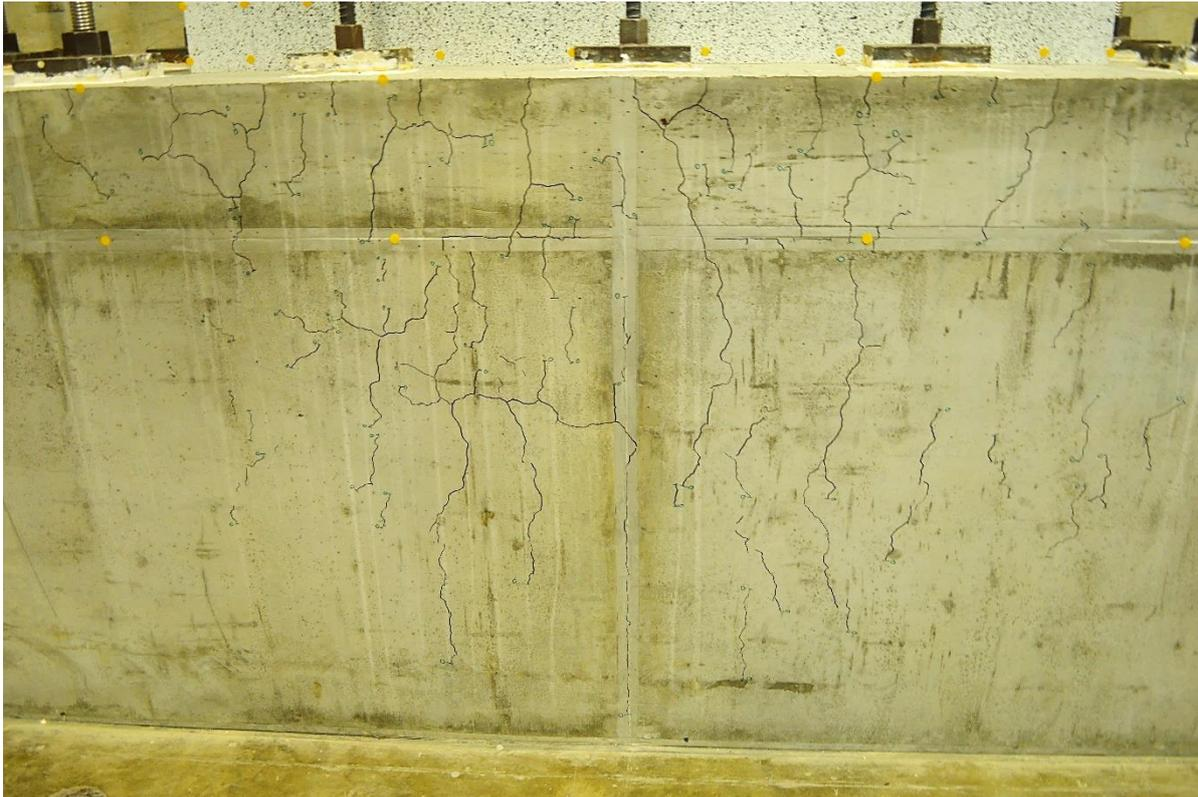
Figure 49 – Shrinkage Cracks observed and marked on the foundation of Test Wall W80C.
