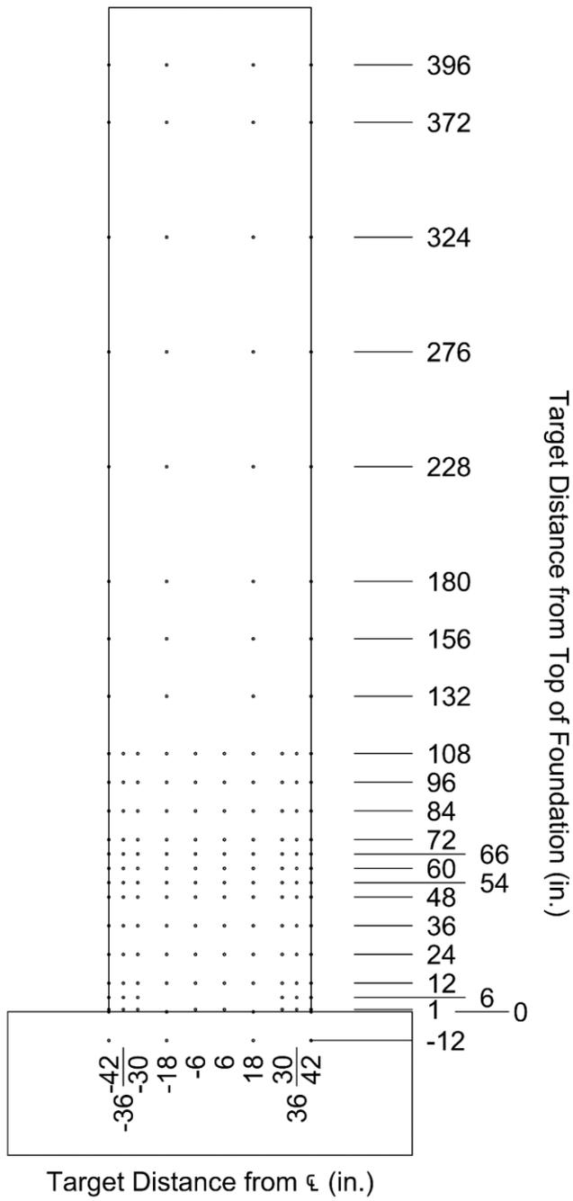
Figure 51 – Layout of Sensors used in Test Walls.
