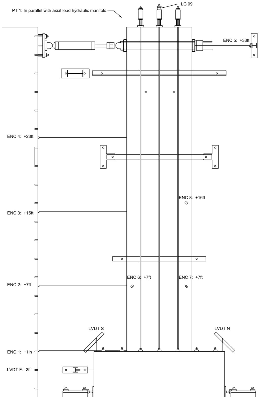
Notes: ENC stands for optical encoder (used to measure displacement), LVDT stands for linear variable differential transformer (used to measure displacement), LC stands for load cell (force transducer), and PT stands for pressure transducer. Both actuators were equipped with a load cell and an LVDT each.
