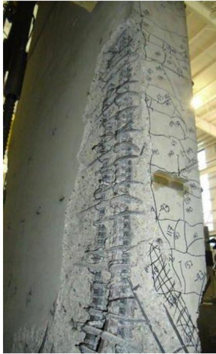
Figure 13 – Splitting in specimen by Villalobos (2014, 2017).
