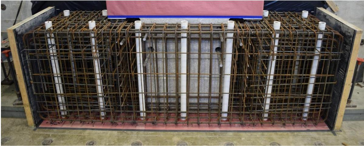
Figure 28 – Reinforcement in Wall Foundation – Side View.
