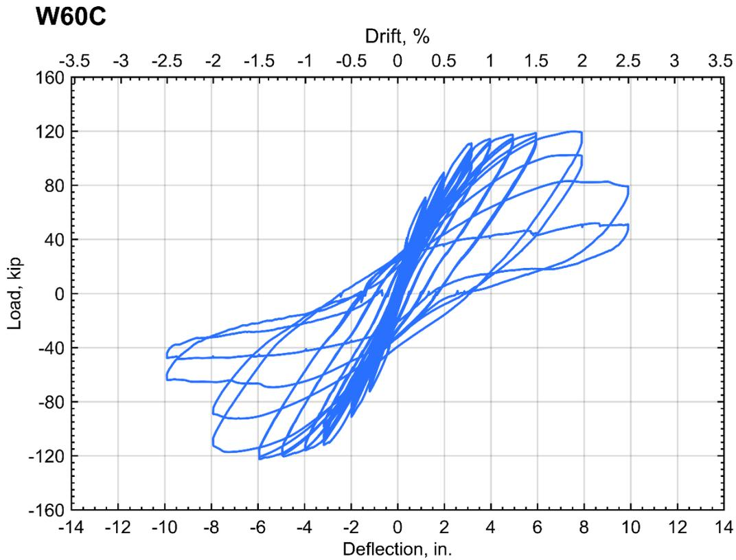
Figure 68 – Specimen W60C, Measured Load-Deflection Curve.
