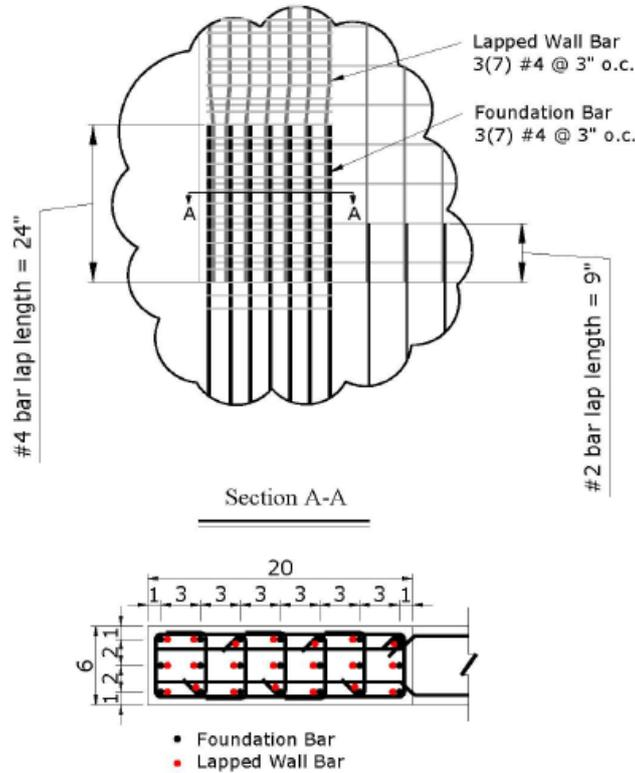
Figure 9 – Typical Splice in Specimens by Birely.
