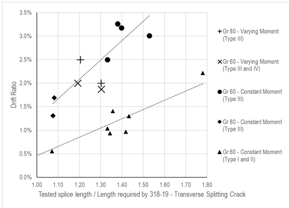
Figure 79 – Variation in Drift Ratio at Failure with Increases in Ratio of Length of Lap Splice to Length Required by ACI318-19 - Formulation Used Assuming Transverse Splitting Controlled.
