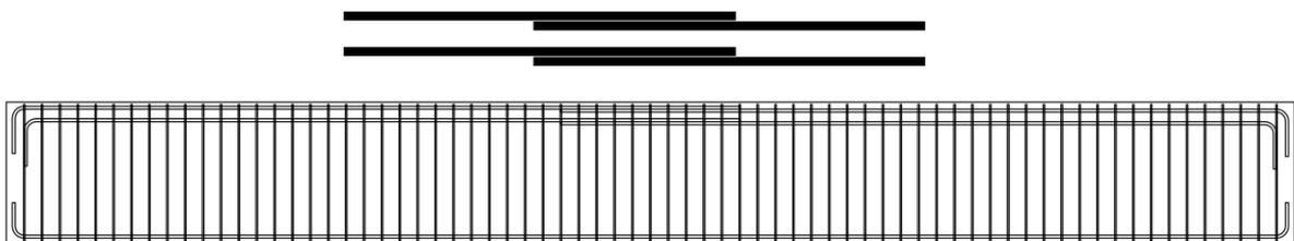
Figure 22 – Lap Splice Configuration B and Typical Beam elevation.
