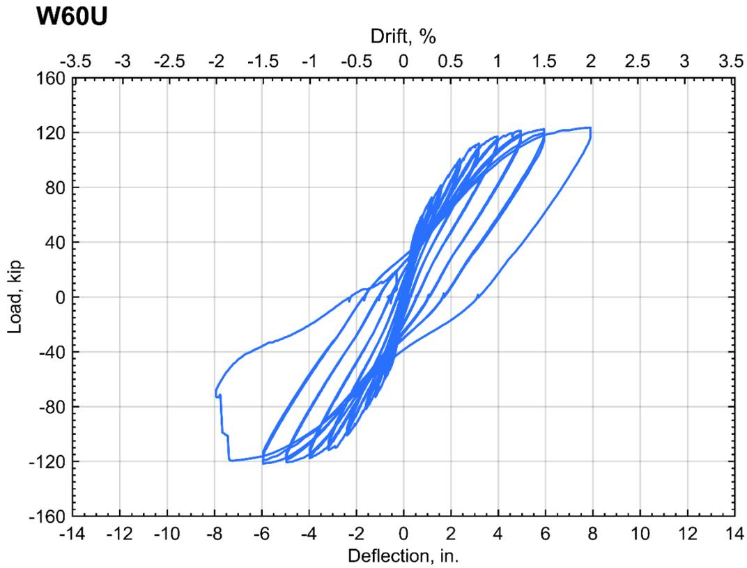
Figure 67 – Specimen W60U, Measured Load-Deflection Curve.
