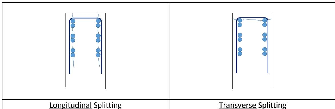
Figure 1 – Illustration of directions of splitting
