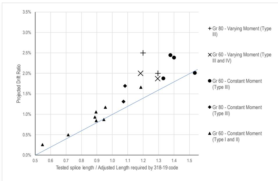
c) drift ratios measured in test beams at failure multiplied by projection factors adjusted in relation to splice length (2/3 for 50 in., 3/4 for 60 in., 1 for 80 in., 0.9 for beams tested by Richter and Hardisty, 2012,2015)
