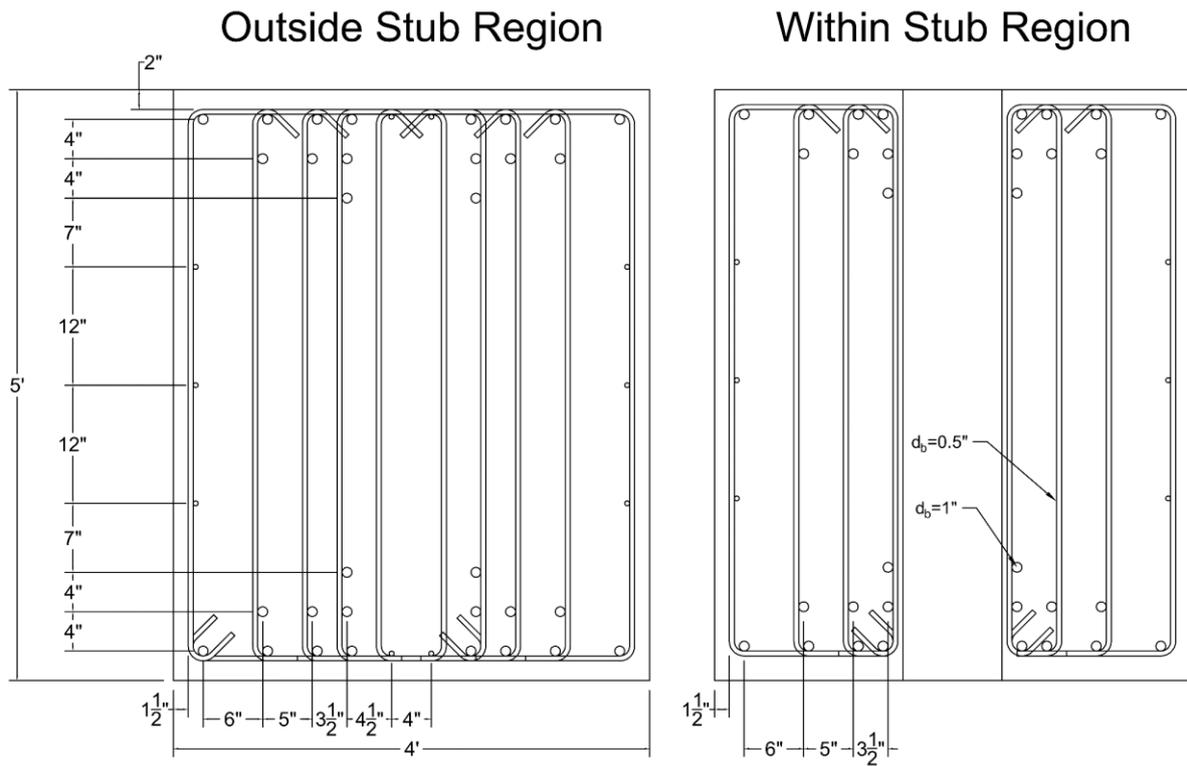
Figure 26 – Cross Sections of Test Wall Foundation.
