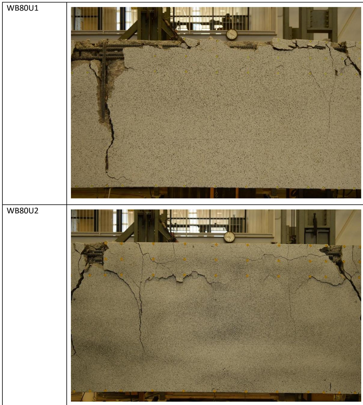
Figure 52 – Photographs Taken after Failures of Test Beams.
