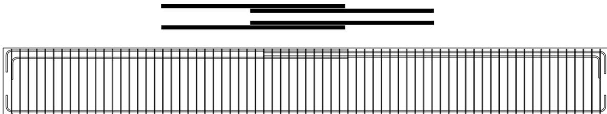
Figure 21 – Lap splice Configuration A and Beam elevation.
