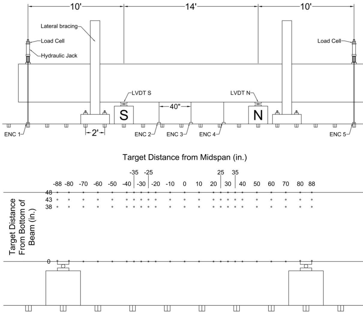
Figure 50 – Layout of Sensors used in Test Beams.
