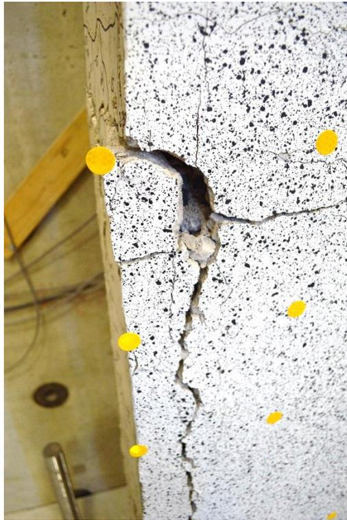
f. W80C Splice Failure (South East Edge)
