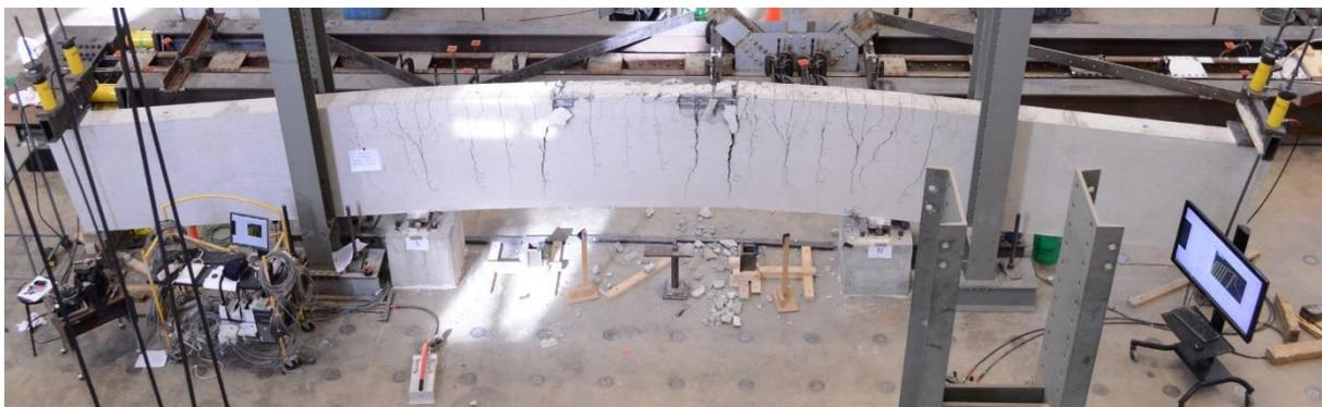
Figure 19 – Four-Point Bending Test Setup – Lap Splice Visible at the Top of the Beam at Midspan.
