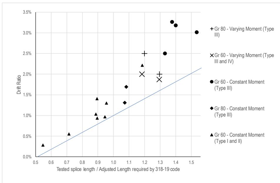
a) drift ratios measured at failure
