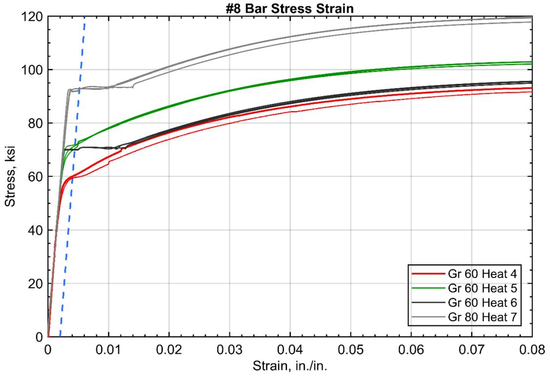
Figure 37 – Comparison of stress-strain curves of longitudinal reinforcement used in this investigation.
