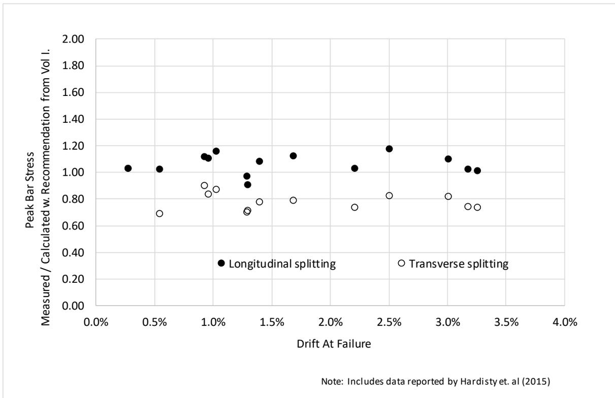
Figure 61<sup>7</sup> – Ratio of Measured to Calculated Peak Bar Stress - Formulation by Fleet et al. (2019).
