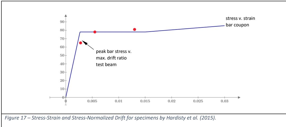
The comparison made also shows that strain is what produced drift, not bond strength (whether expressed as bond stress or as stress in the bar). Understanding that the capacity of a structural system to resist earthquake demands is often expressed better in terms of drift, the example above suggests that the data from bond tests need to be re-examined in terms of strain or some measure of deformability, not stress only.
