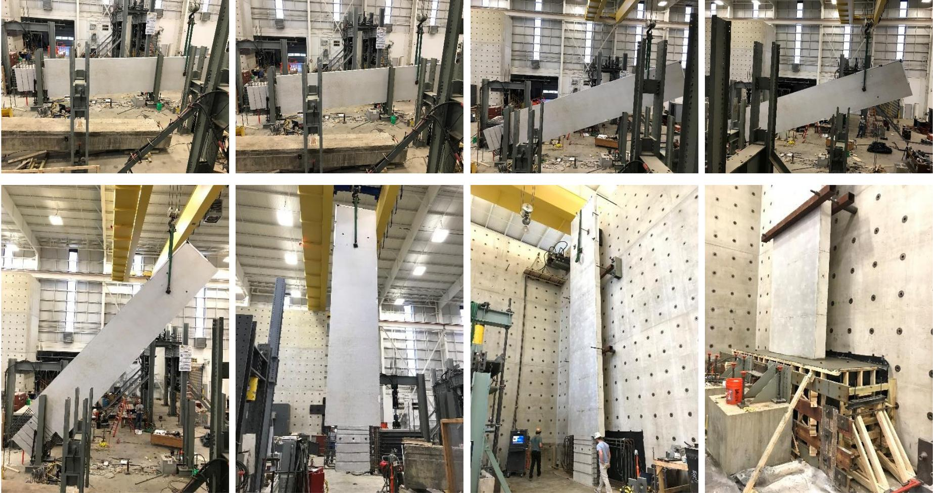
Figure 47 – Wall tilting process and foundation fabrication.
