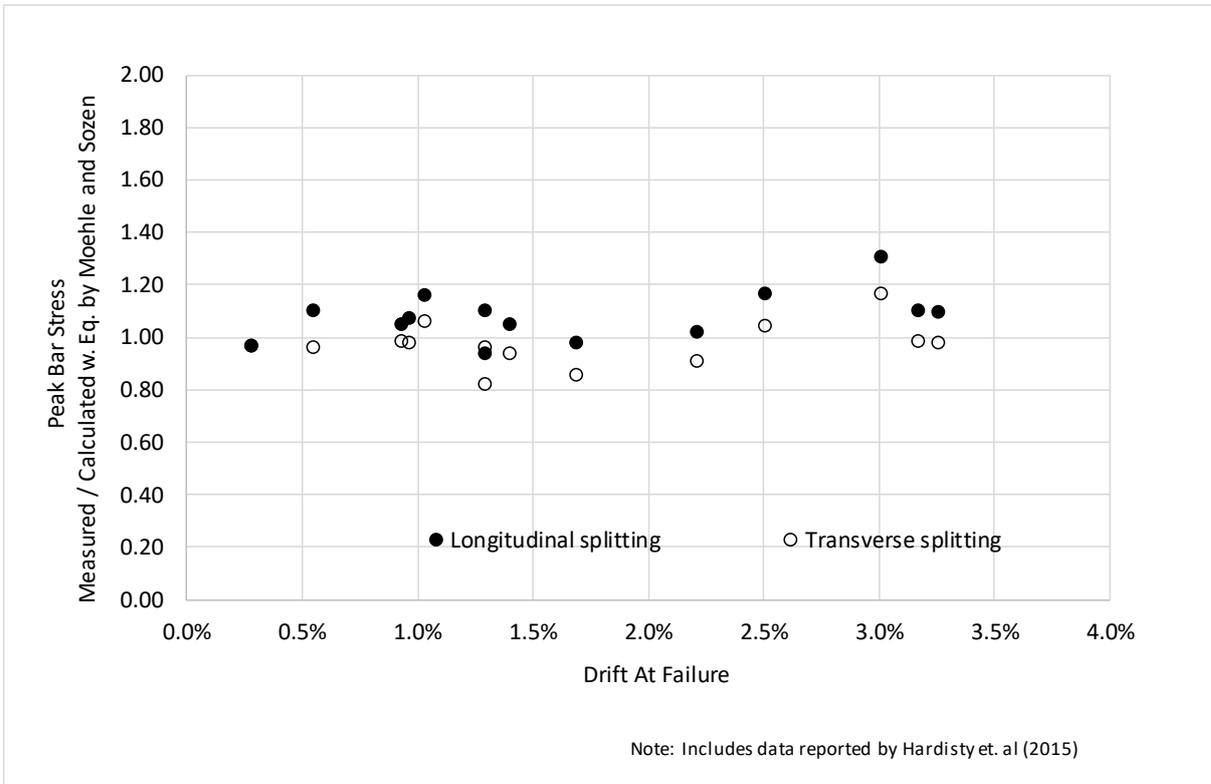
Figure 59<sup>6</sup> – Ratio of Measured to Calculated Peak Bar Stress - Formulation by Sozen and Moehle (1990).
