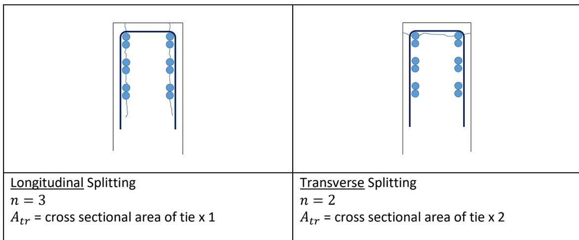
Figure 57 – Illustration of assumed directions of splitting and examples of choices for parameters  $n$  and  $A_{tr}$ .
