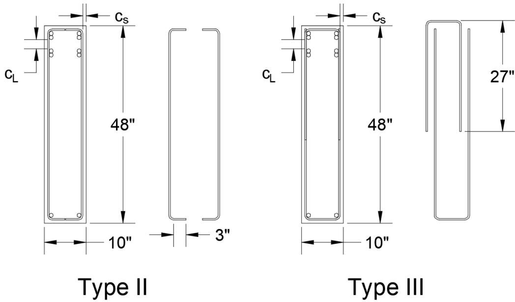
Figure 20 – Typical beam cross sections and Transverse Reinforcement Detailing. See Table 2 for Descriptions and Values for  $C_L$  and  $C_S$ .
