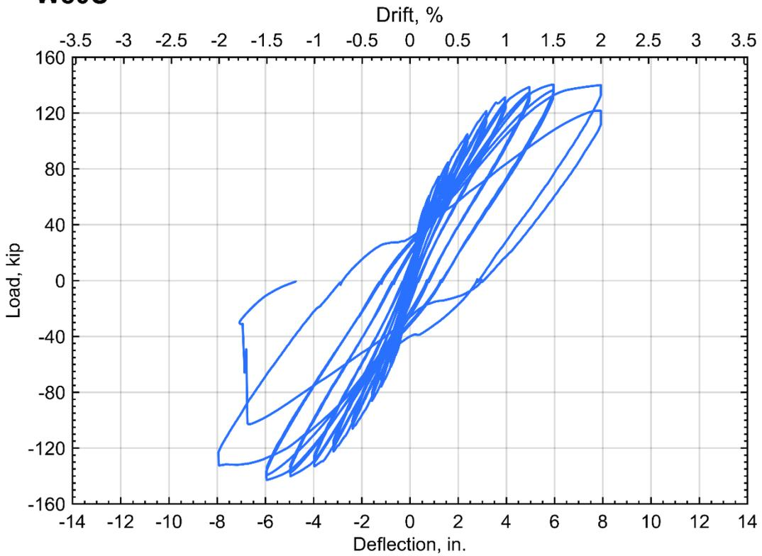
Figure 69 – Specimen W80U, Measured Load-Deflection Curve.
