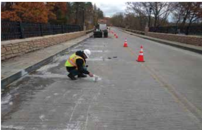
In a recently completed study funded by the ACI Foundation, samples of GFRP bars were collected from bridge decks
