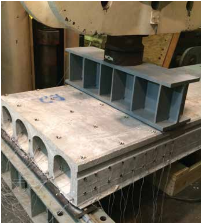
Setup for hollow-core slab testing (photo courtesy of Gustavo J. Parra-Montesinos)
