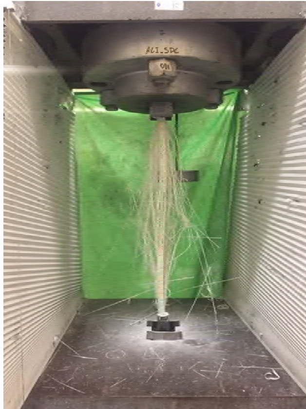
Fig. 54—Pristine GFRP tension failure
