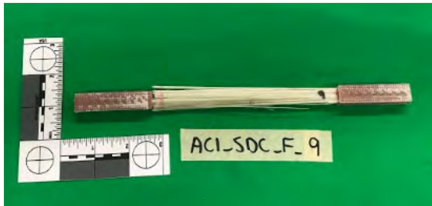
Fig. 47. Coupon F_9 after failure
