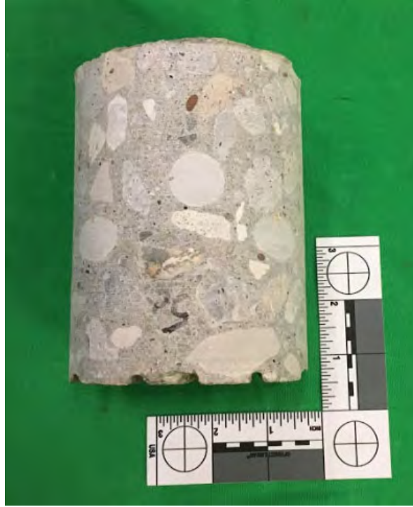
Fig. 36–Cuyahoga Bridge core sample
