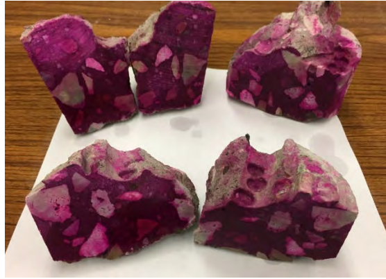
Fig. 13. Cuyahoga carbonation depth results -S&T
