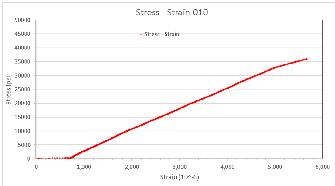
Fig. 67. Stress strain curve for bar 010
