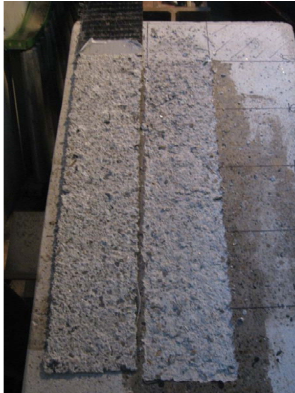
Figure 4.17 Failure of specimen F2-0a-24
