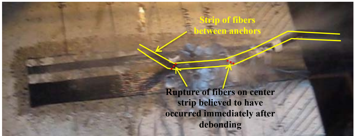
Figure 4.9 First frame from test video of specimen S1-4a-1-24 showing failure
