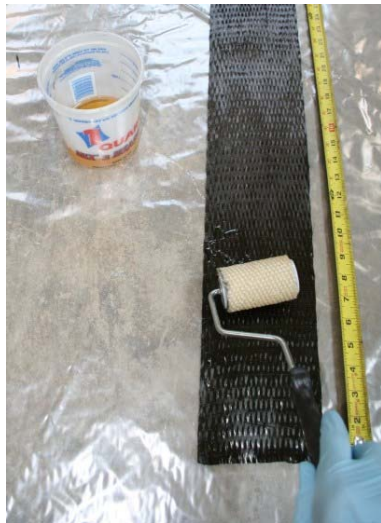
Figure 3.9 (a) The two component epoxy is mixed with a mixing paddle attached to a drill and (b) epoxy is applied to the surface as a surface primer
