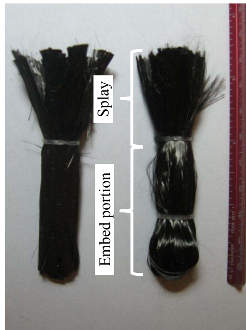
Figure 3.5 Handmade Sika anchor (Left), Fyfe anchor (Tyfo® SCH Fibr™ Anchors) (Right)
