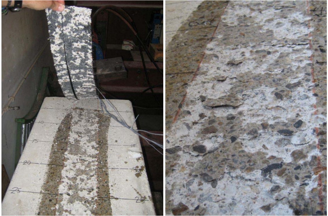
(a) (b) Figure 4.4 Specimen S1-0a-24 after failure
