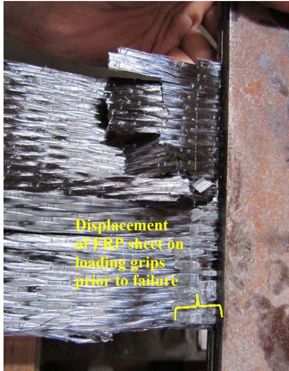
Figure 4.13 Fibers on right side of specimen S1-4a-2-24 slipped on loading plates prior to failure (note picture is after failure)
