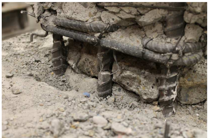
Figure 3.3.4: Failure Mechanism of SBM100 by Fracture of Longitudinal Bars
