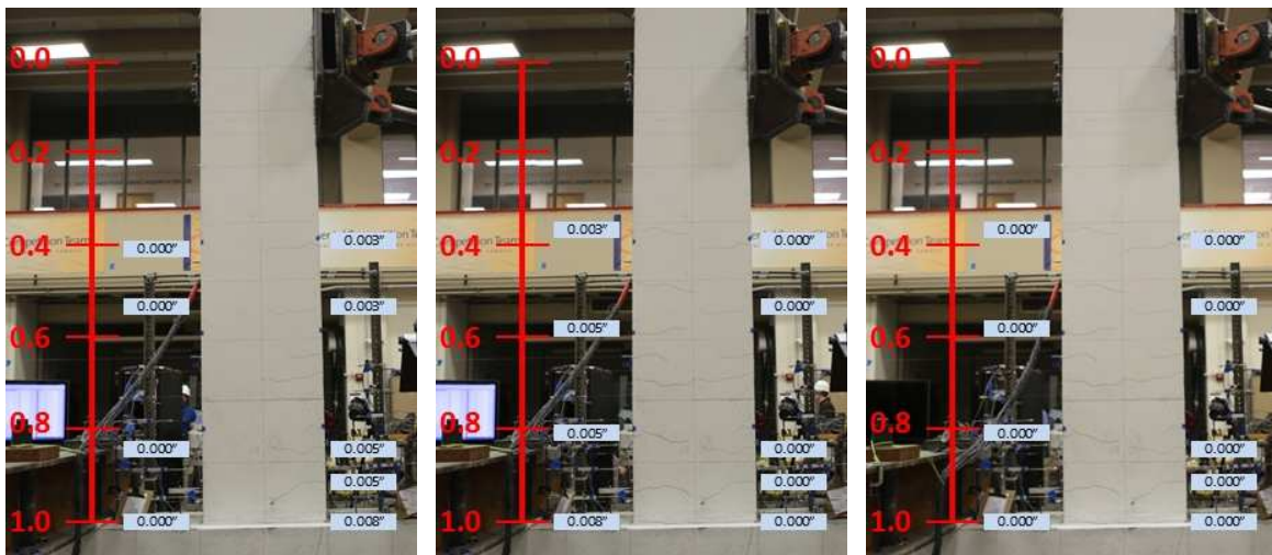
Figure C-1: Measured Crack Widths at Drift Ratio of 0.35% – Specimen SBH60
