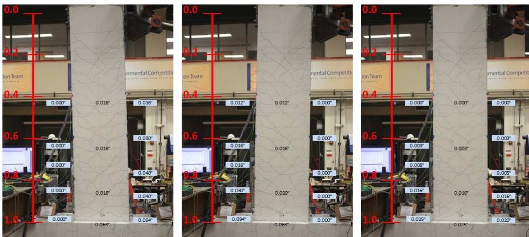
Figure C-27: Measured Crack Widths at Drift Ratio of 2.45% – Specimen SBM100
