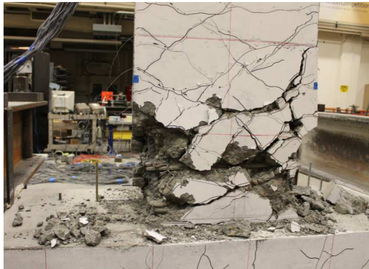
Figure 3.3.1: Failure Mechanism of SBH60 by Twisting of Beam (Global Instability)
