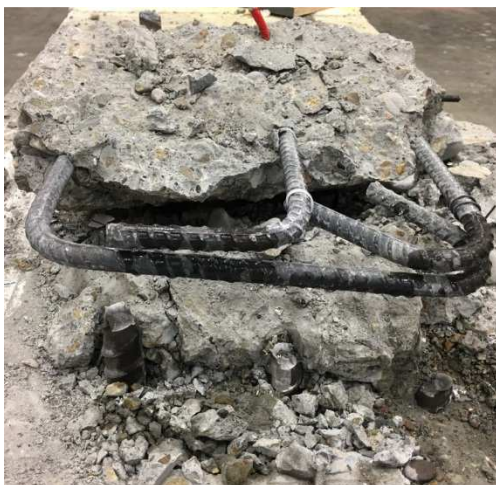
Figure 3.3.4: Failure Mechanism of SBM100 by Fracture of Longitudinal Bars
