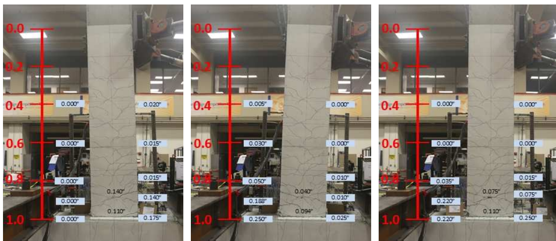
Figure C-14: Measured Crack Widths at Drift Ratio of 3.45% – Specimen SBH100
