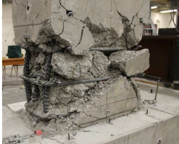
Figure 3.3.2: Failure Mechanism of SBH100 by Buckling of Longitudinal Bars Over Several Hoop Spacings
