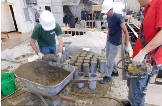
**Figure 2.20: Making of Cylinders**
