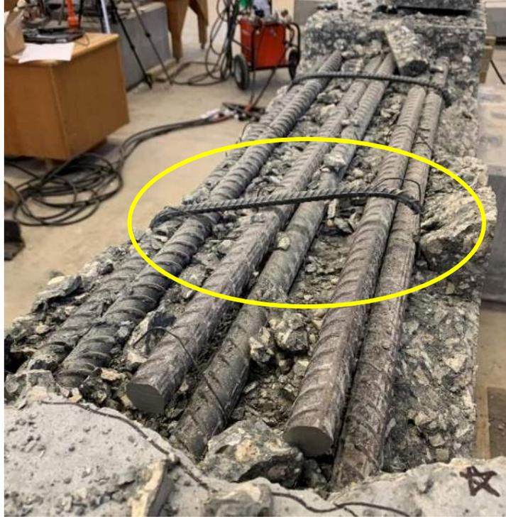
**Figure 4.58: Ruptured Stirrup on Specimen C3/60/2-40-10-50**
