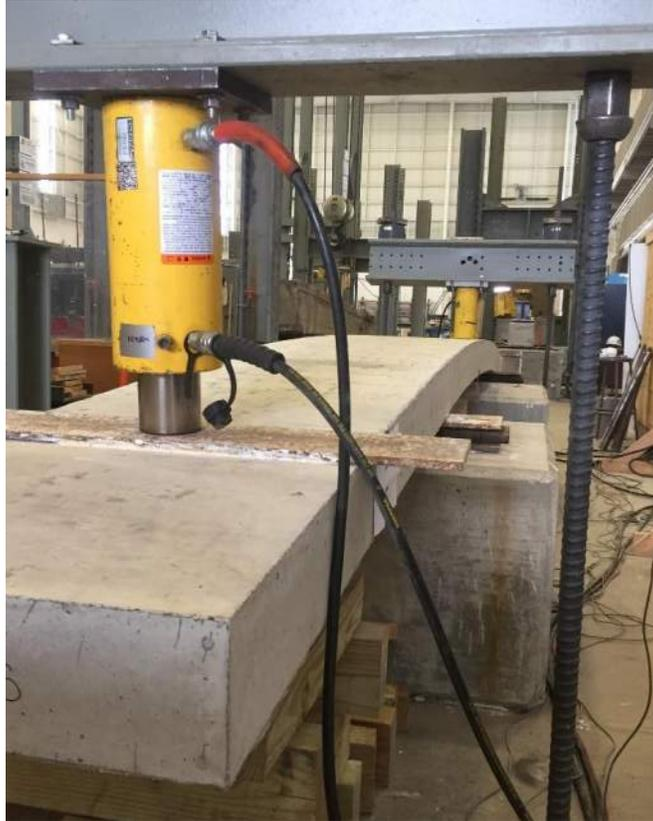
**Figure 3.35: Slab Deformation during Testing (S-100-5)**
