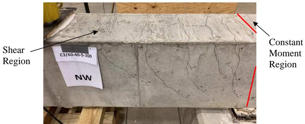
**Figure 4.48: Shear Span – Late Testing (C3/60-40-5-200)**
