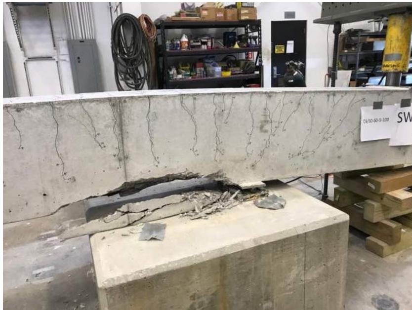
**Figure 2.37: Flexural Failure (C4/60-60-5-100)**
