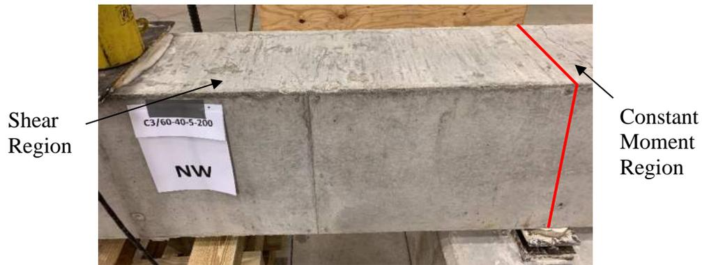
**Figure 4.47: Shear Span – Early Testing (C3/60-40-5-200)**
