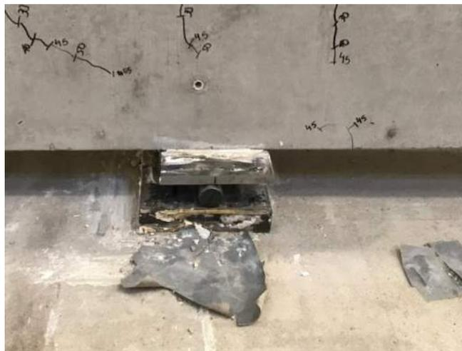
**Figure 2.26: Roller-Roller Support (U-120-5-M)**
