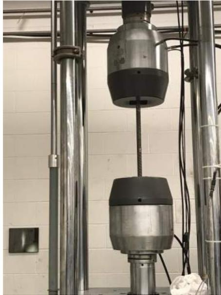
**Figure 2.7: Testing of No. 8 Bars**
