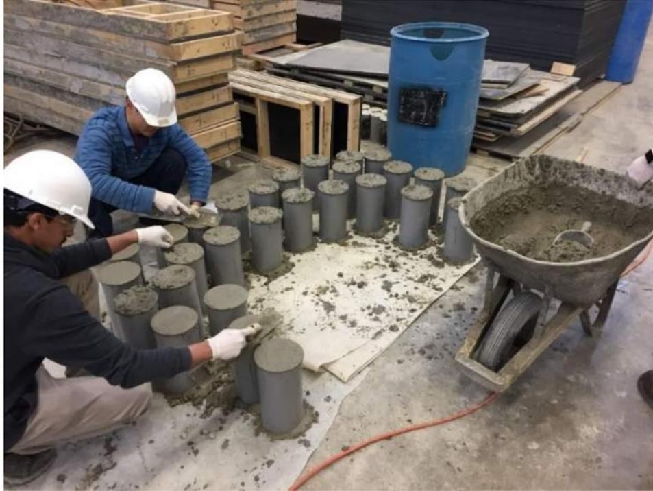
**Figure 3.15: Series V Cylinder Casting**
