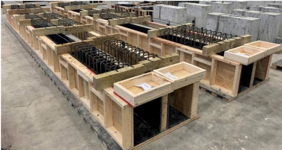
**Figure 4.16: Series VII Cage Support Blocks**
