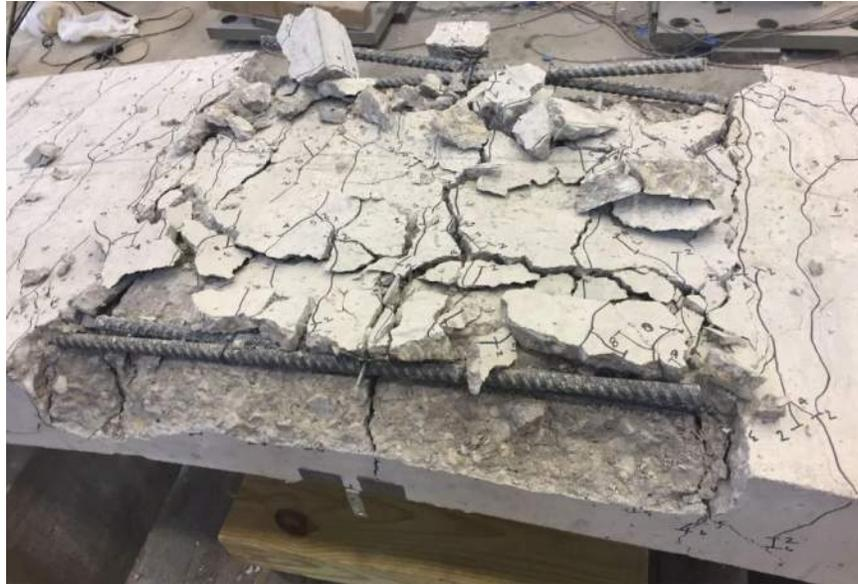
**Figure 3.45: S-40-5 Face- and Side-Splitting Failure**
