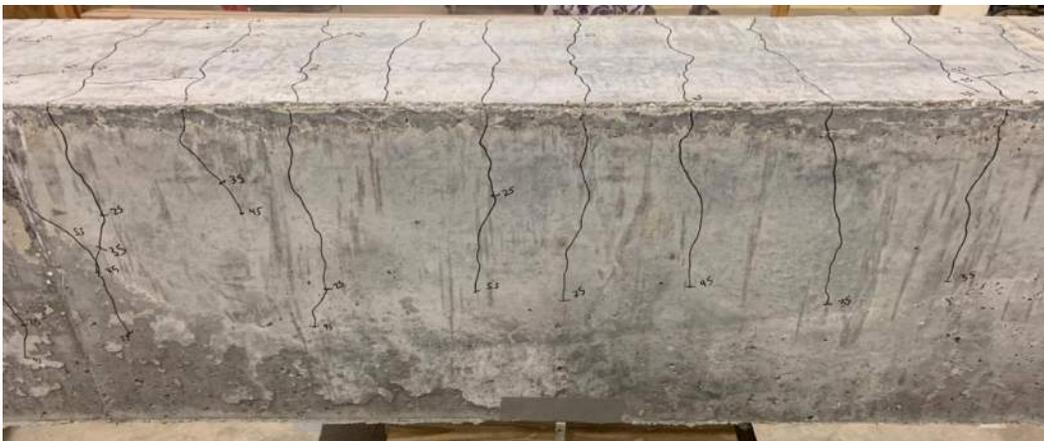
**Figure 4.39: Typical Flexural Cracking within Unconfined Splice Region (U-60-10)**
