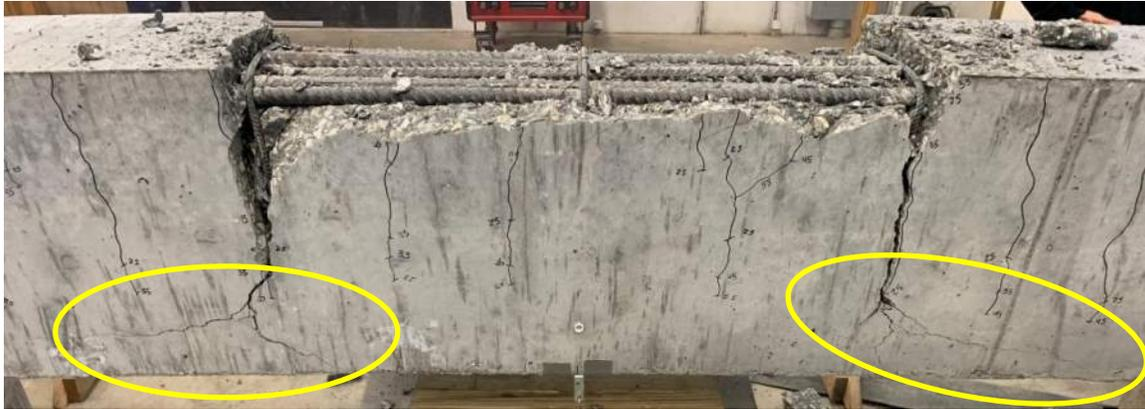
**a) Full Splice at Failure**
