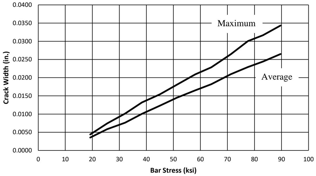
**Figure 2.40: Comparison of Average and Maximum Crack Widths**
