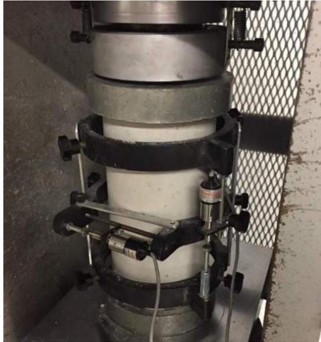
**Figure 3.8: Series V Modulus Testing Setup**
