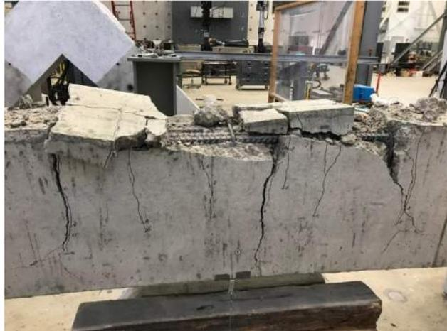
**Figure 2.36: Typical Confined Specimen Failure (C3/60-40-5-100)**
