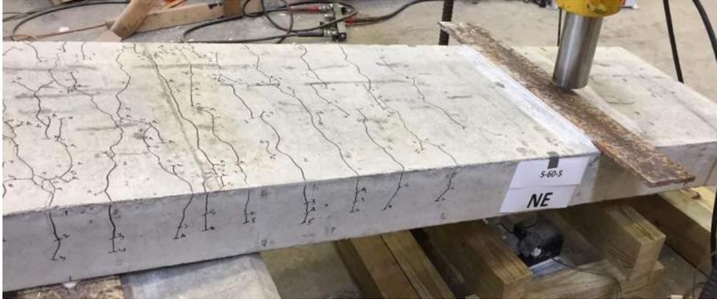
**Figure 3.42: Post-Failure Shear Span Cracking (S-60-5)**
