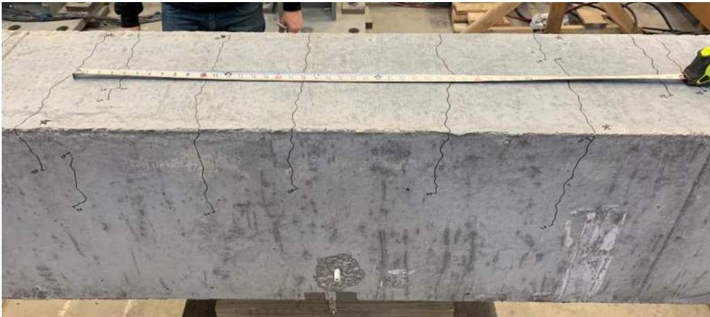
**Figure 4.45: Transverse Flexural Cracking within Splice Region (C3/60/2-40-10-50)**
