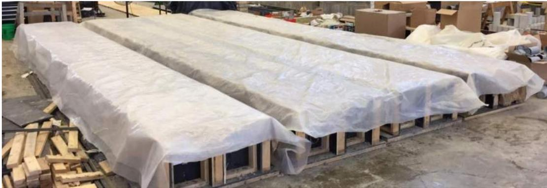
**Figure 4.29: Series VI Moist Curing – Plastic Cover**
