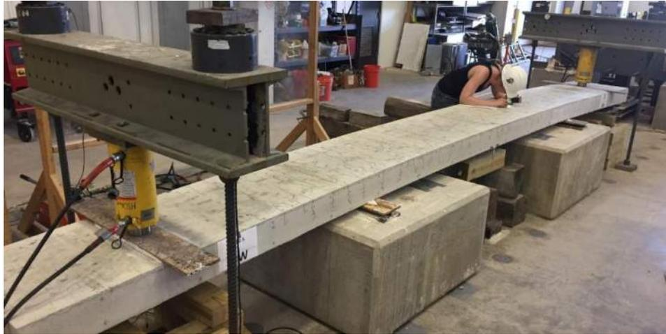
**Figure 3.32: General Slab Test – Crack Mapping (S-80-5)**
