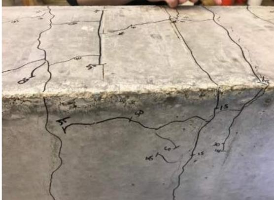
**Figure 2.33: Longitudinal Cracking in Unconfined Specimens**
