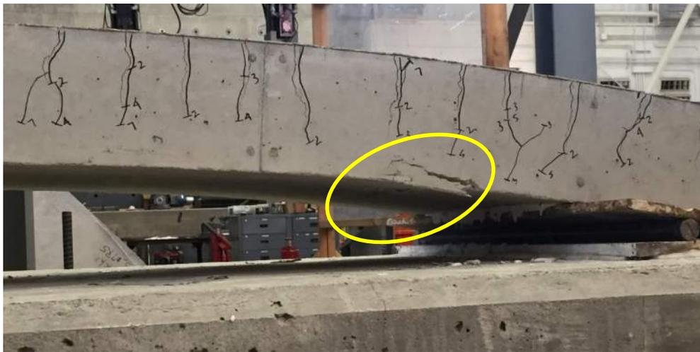
**Figure 3.50: Initiation of S-80-5 Failure – East Elevation**
