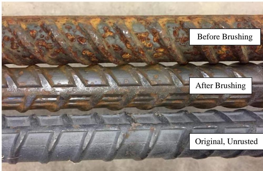
**Figure 4.12: Comparison of Grade 100 Bar Surfaces**
