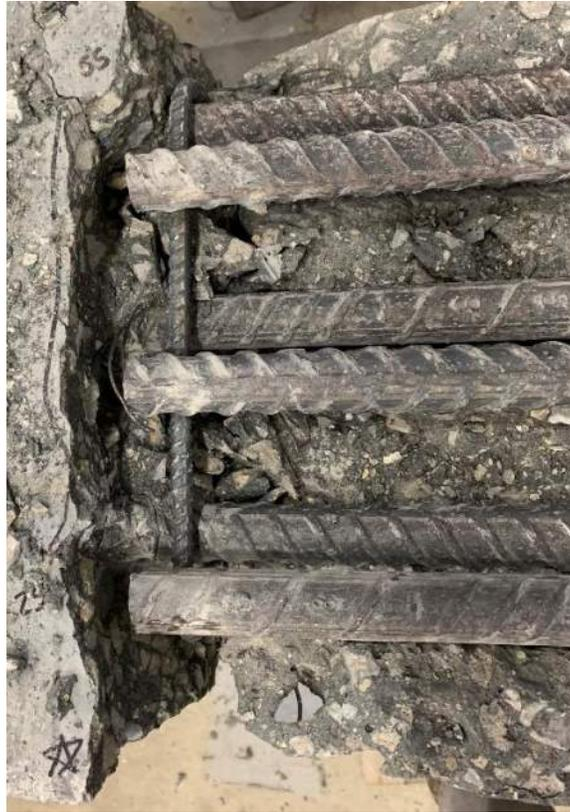
**Figure 4.56: Bar Slip on Specimen C3/60/2-40-10-25**
