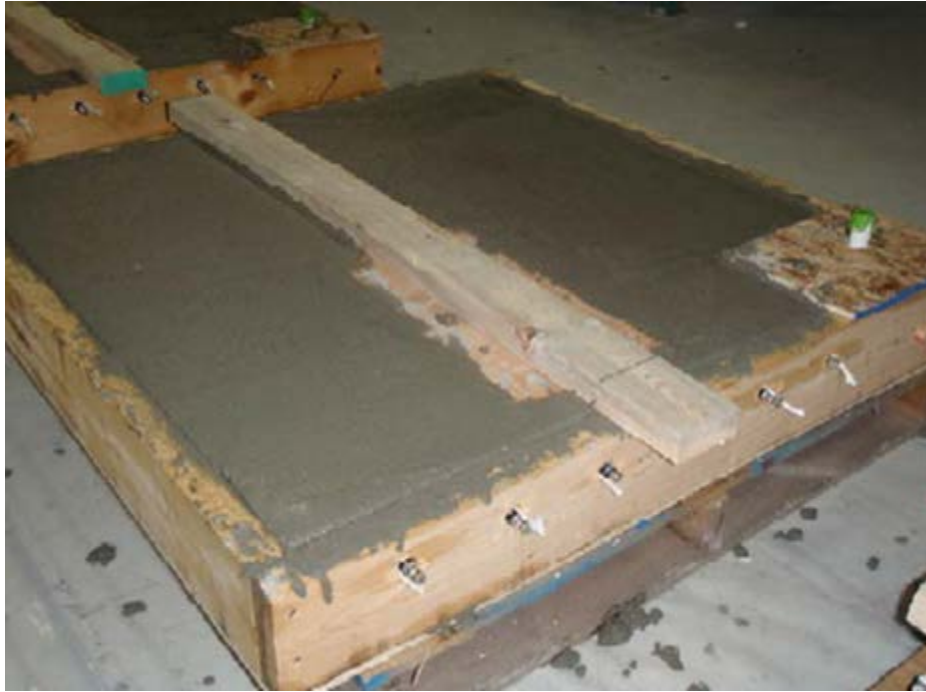
Figure 4 – Block attached to mold to create area of reduced concrete cover. The area of reduced cover makes a hotspot.
