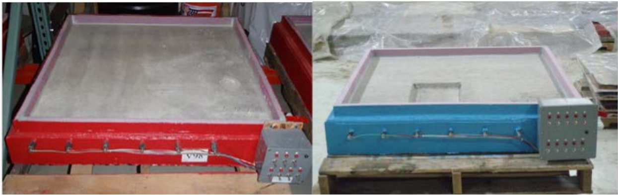
Figure 10 – Example of a Configuration A slab (left) and Configuration B slab (right) ready for use.
